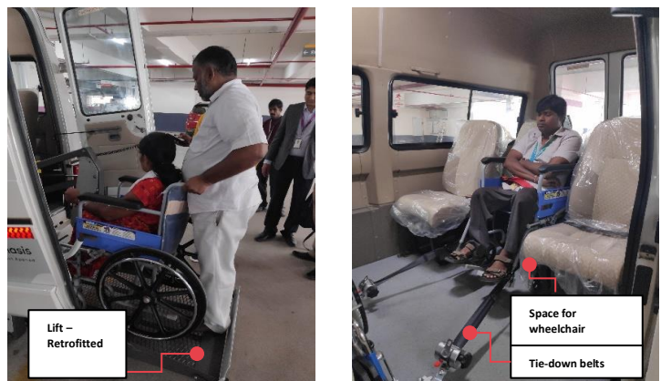
Figure 1: Retrofitted features in Uber Access
