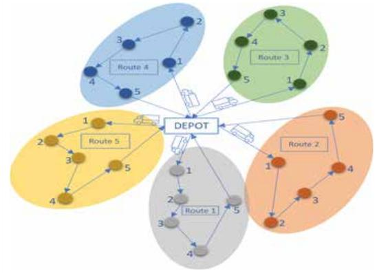
The route optimization engine has a two-fold task. Firstly, assignment of packages to vehicles within a given fleet and secondly, generate the order of deliveries for each vehicle in the fleet, based on pickup and deliveries schedule of a package from a single depot. The optimization engine minimizes the overall distance covered and hence the cost while managing the problem constraints.
