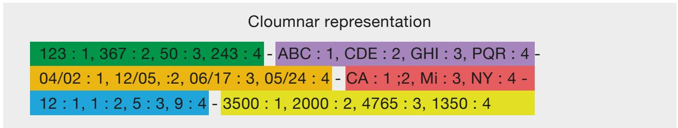
One of the advantages of this representation is the possibility to compress data. Row 1 and 2 has same value for state columns i.e., 'CA'. Below columnar representation compresses both values as shown in the circle.
